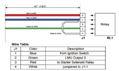
4. Connect the Green wire from the starter relay to the green wire coming from the device's wires. If there are two green wires, it is pin 2 (20-wire harness only)
